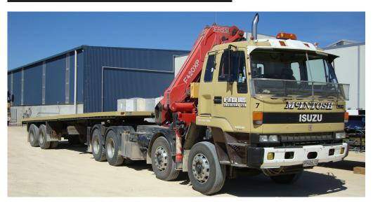
This unit can change between a flat deck truck and a tractor unit
